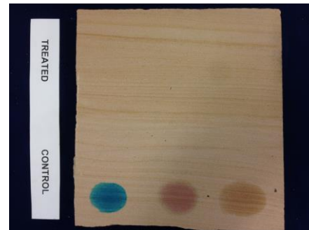
Stains removed, washed and dry
