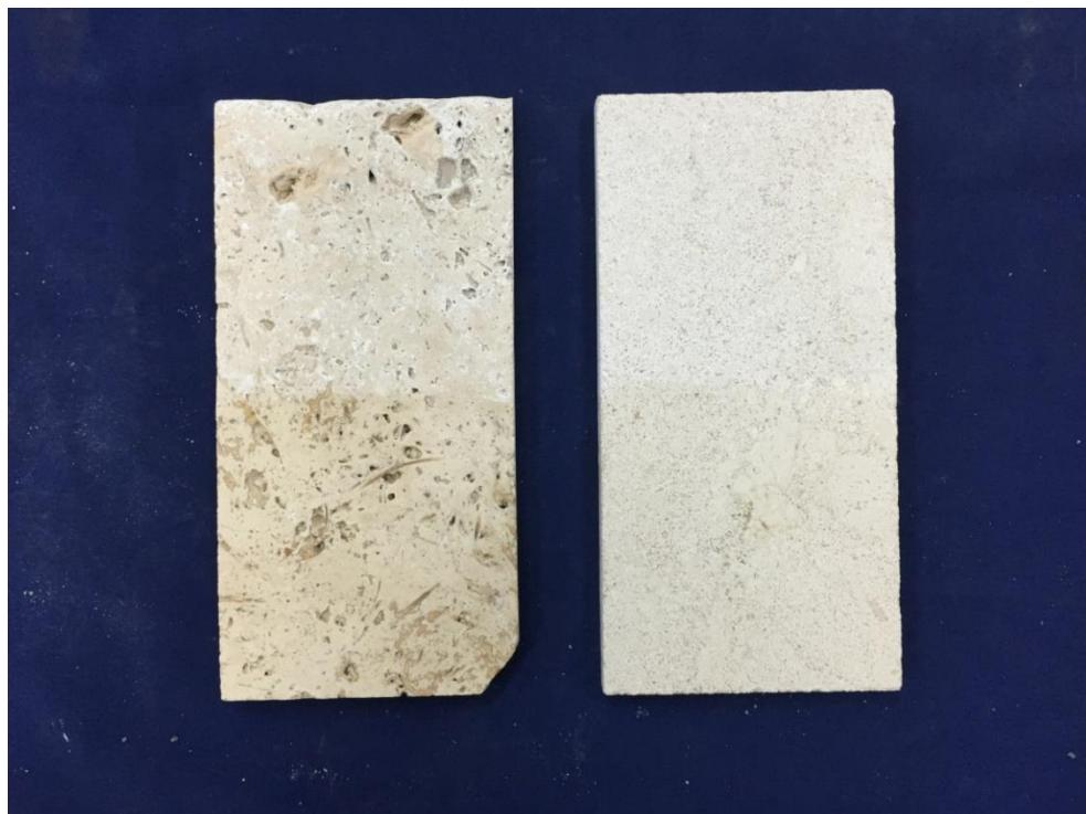
4. Concrete: wet cast pavers and pressed pavers
