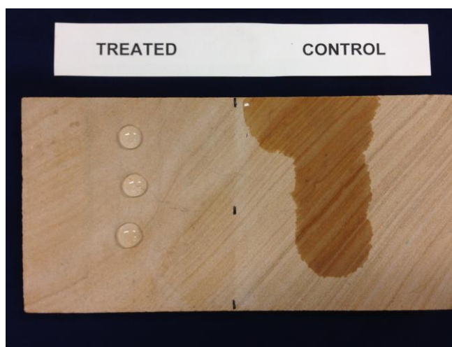
Figure 1. Surface Beading Achieved by Emulsion GPE50P
