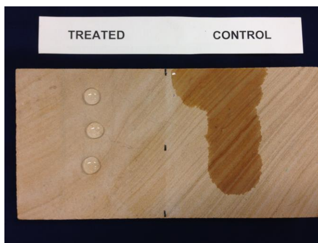
Figure 1. Surface Beading Achieved by Emulsion GPE50P
