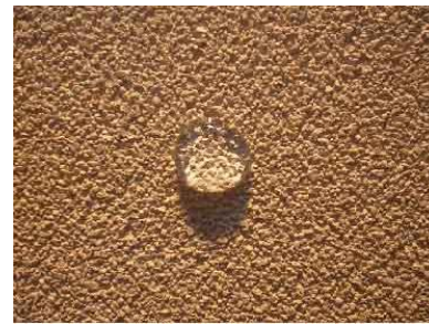
Textured Coating with ADM80-1: It shows excellent beading effect of water droplet
