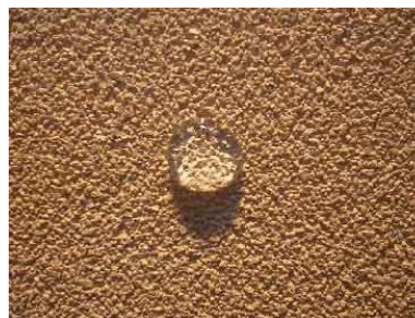
Textured Coating with ADM80-1: It shows excellent beading effect of water droplet
