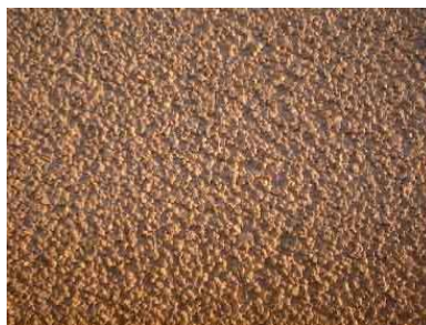
Standard Textured Coating: The water droplet is absorbed through the coating
