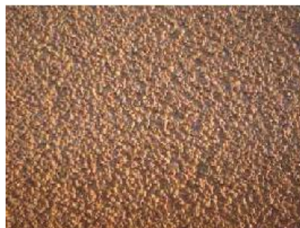
Figure 1. Excellent beading effect of earth render surface
