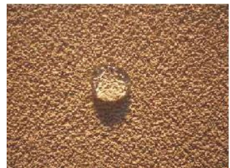
Figure 1. Excellent beading effect of earth render surface
