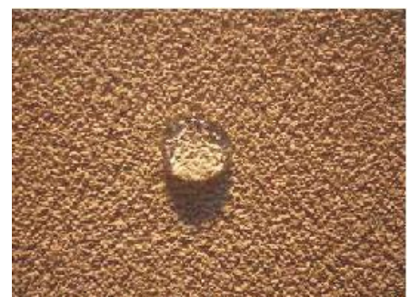
Figure 1. Excellent beading effect of earth render surface
