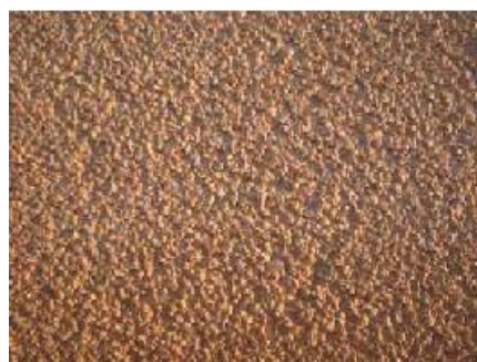
Figure 1. Excellent beading effect of earth render surface
