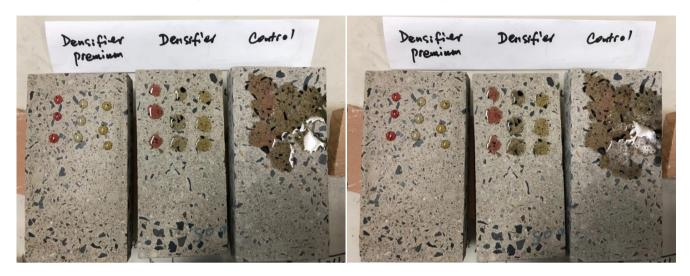
Substrate finished with 800 grit resin pad (left photo: 1 hour and right photo: 24 hours)
