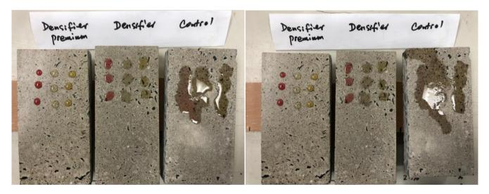
Substrate finished with 70 grit metal pad (left photo: 1 hour and right photo: 24 hours)
