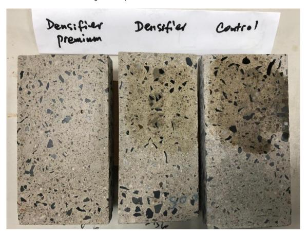
Substrate finished with 800 grit resin pad
