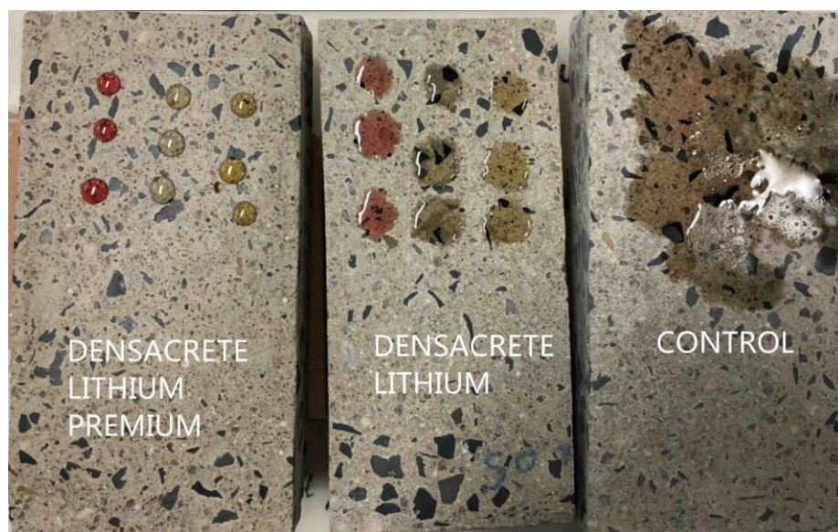
Figure 3. Oil beadings (engine oil, olive oil & heavy engine oil) after 24 hours
